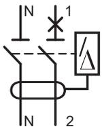
**en** Residual Current Circuit Breaker with Overcurrent Protection (RCBO) provides:
